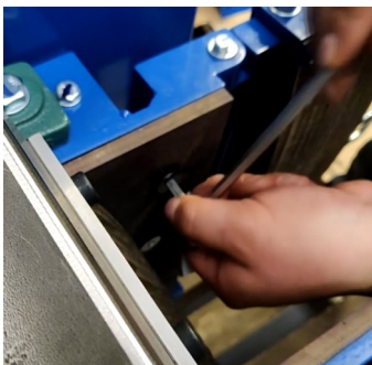
Attach the second side liner with the correct screws
