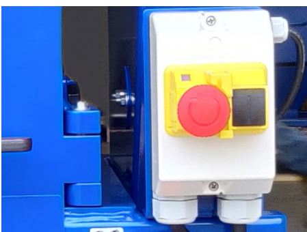
Use the control box to start and stop the machine
