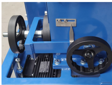
Use the lever to adjust the gap
