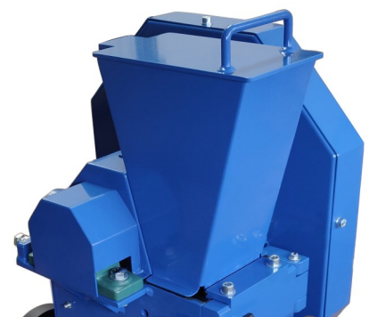
Place the sample in the feeder
