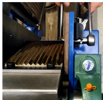
Use the wrench tool to easily attach the side liner
