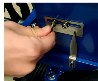
Set the measurements to zero and attach the measurement plate once again
