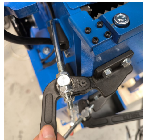
3. Use the upper handle to open the door by pushing inwards
