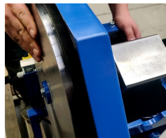
Remove the cover and move the crusher to it's highest position
